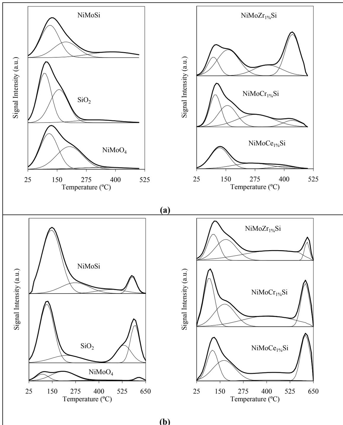
**Fig. 1.** Thermograms obtained by TPD-NH<sub>3</sub> (a) and TPD-CO<sub>2</sub> (b) for the unsupported NiMoO<sub>4</sub>, the SiO<sub>2</sub> support, and the silica supported NiMoO<sub>4</sub> catalysts
